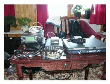
My setup was ICOM 706 MK2G, LDG Z-11 Pro Tuner, Signal link SL-1 sound card interface, random wire antenna, MFJ 33 foot push up mast and HP Omni book laptop. I worked most of Europe, West Asia, Middle East and some DX stations. I worked Siberian and North American East Coast stations. Propagations were pretty good and bands were open almost the whole day and night, but unfortunately not very good for communication with California.
